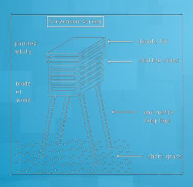
To ensure an accuracy of measurement of air temperature, the thermometers are mounted in a box of approved pattern called as the 'Stevenson's screen'.
